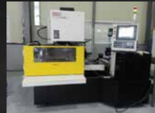
Wire Cutting Machine
