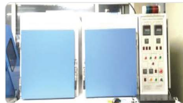
VALVE ASS`Y Reliability Test - Cooling resistance test : 96HR left at lowtemperatures - Thermal shock test : low => normal => high=> normal- temperature 20 CYCLE test
