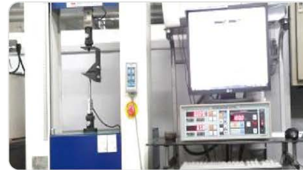
VALVE ASSY Reliability Test - TORQUE test
