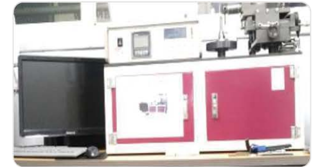
VALVE ASS'Y Reliability test - Spring TORQUE Rig test
