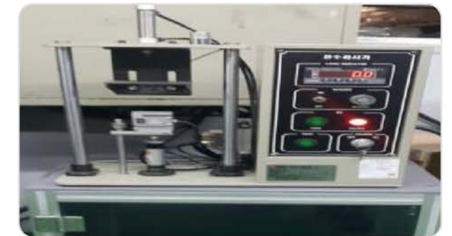
VALVE ASS'Y Reliability test - Tension & Compression test
