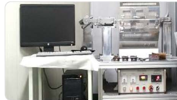
VALVE ASS'Y Reliability Test - At 550 °C, 40,000 CYCLE (open /close) -1 CYCLE (open/close) in every 2 seconds
