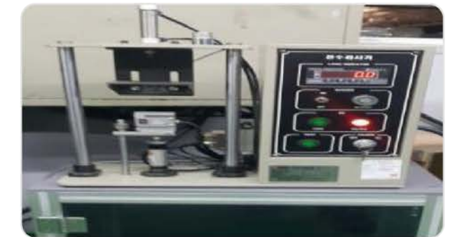
VALVE ASS'Y Reliability test - Tension & Compression test
