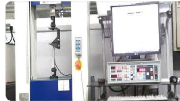
VALVE ASSY Reliability Test - TORQUE test
