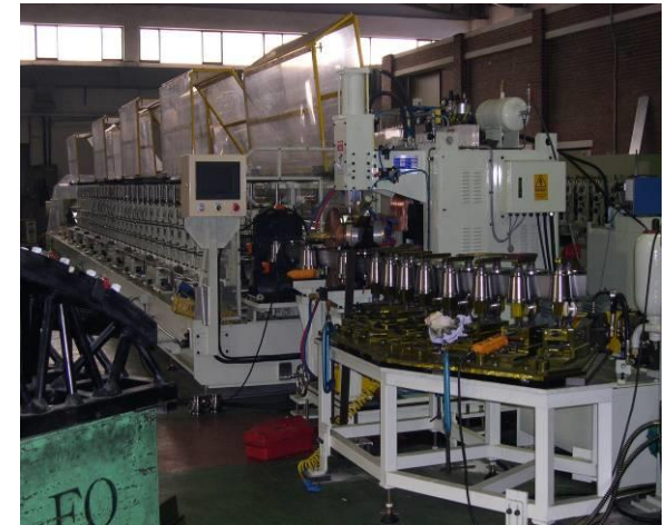
DONG WON NFA-CAR ROLL FORMING MACHINE \phi 45X35
