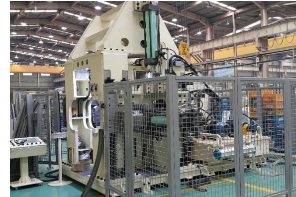
SUNGWOO(1, 2, 3 LINE) BUMPER STRETCH BENDING M/C
