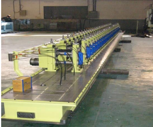
JAPAN TOYOTA \phi 65X35ST ONE BASE CASSETTE (BUMPER LINE)
