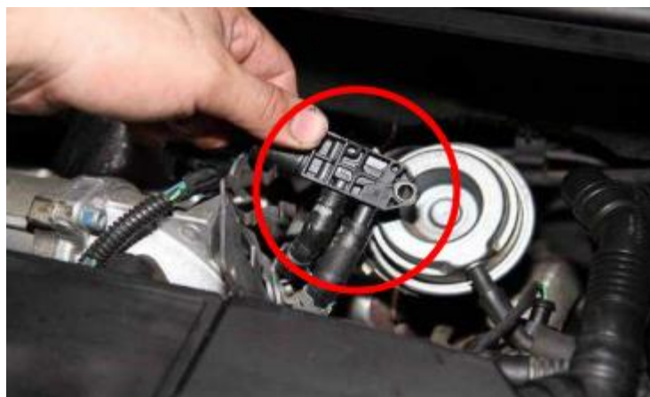
DPF sensor (Exhaust Gas Pressure sensor)
