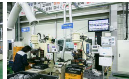
Welding Line (Fool Proof)
