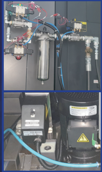
C-Jet Coolant Supply System
