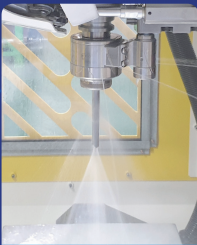
C-Jet Pressurizing Oil Hole Spray
